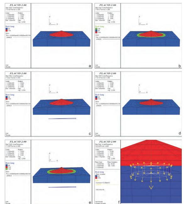
Figure 1. The five studied model geometries (a-e) and a wireframe outline of the defined region of the pressures source (f)
