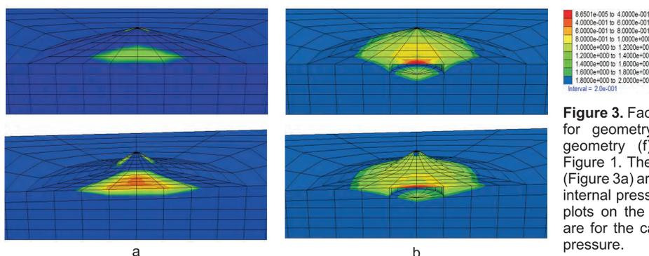
Figure 3. Factor of safety plots for geometry (a) (top) and geometry (f) (bottom) from Figure 1. The Plots on the left (Figure 3a) are for a case of no internal pressurisation and the plots on the right (Figure 3b) are for the case of a 20 MPa pressure.
