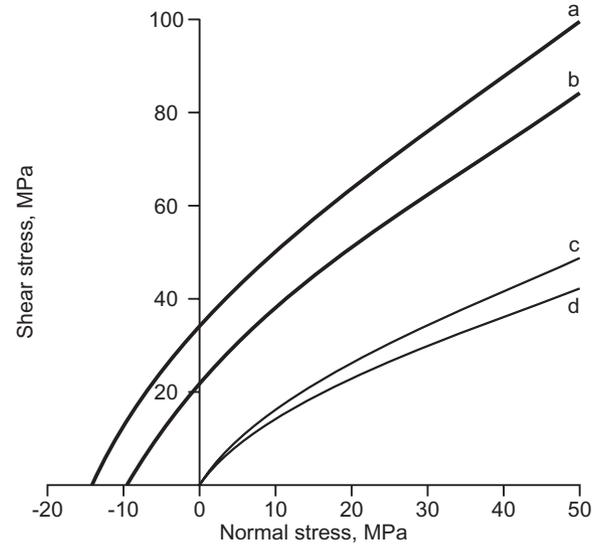
**Fig. 4.** Mohr failure envelopes for intact rhyolite and a rhyolitic rock mass using relevant values from Hoek & Brown (1981). Intact:  $m_i = 16$ ,  $s = 1$ ,  $\sigma_c = 225$  MPa (curve a); curve b is as curve a, but  $\sigma_c = 150$  MPa. Rock mass:  $m = 2.68$ ,  $s = 0.0039$ ,  $\sigma_c = 225$  MPa (curve c); curve d is as curve c, but  $\sigma_c = 150$  MPa. The Hoek–Brown constants  $m$  and  $s$  were determined from equations (2) and (3) using an RMR of 50.
