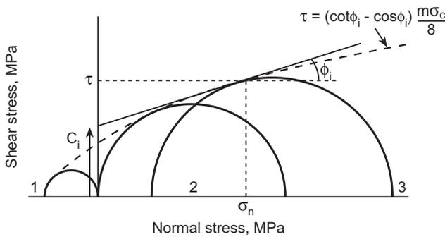
**Fig. 3.** Typical failure circles for rock and the Bray strength envelope (Hoek 1983): 1, uniaxial tension; 2, unconfined axial (uniaxial) compression; 3, confined (triaxial) compression. Also shown are the instantaneous values of angle of friction ( $\varphi_i$ ) and cohesion ( $c_i$ ).
