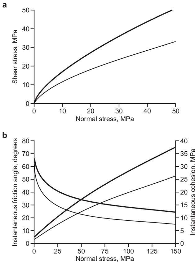
**Fig. 7.** (a) Mohr failure envelope and (b) instantaneous friction angle and instantaneous cohesive strength, for a rock mass where  $\sigma_c = 150\text{MPa}$ ,  $m_i = 15$ ,  $RMR = 65$  and  $D = 0$  (bold line) or  $D = 1$  (fine line).
