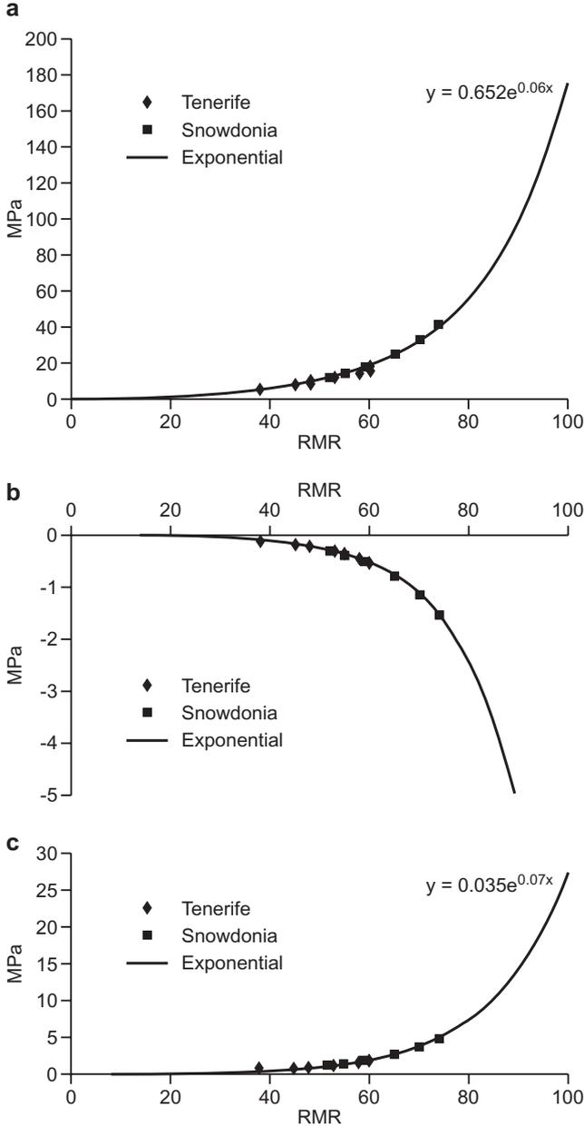
**Fig. 2.** Dependence of rock-mass compressive (a), tensile (b) and cohesive (c) strength on RMR for lavas (basalt, phonolite and rhyolite) from Snowdonia and Tenerife. An exponential best-fit curve has the form  $\sigma_{cm} = 0.652^{(0.06\text{RMR})}$ . This predictive relationship also appears to hold true for the rock-mass tensile and cohesive strengths.
