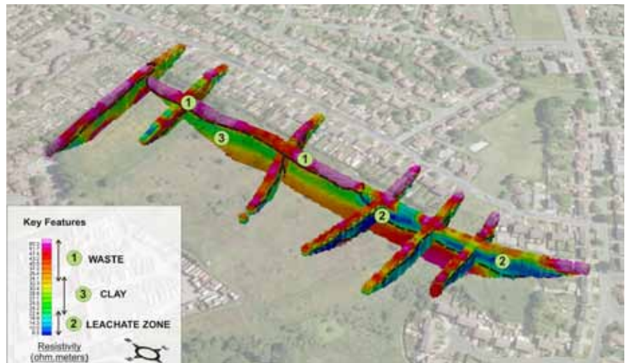
Resistivity profiles across a closed landfill site
