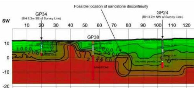
Seismic refraction data revealed variations in the bedrock, and the properties of shallow made ground
